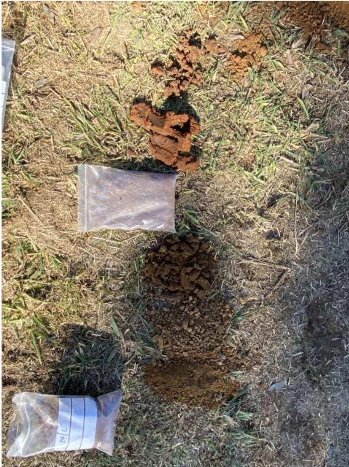
Figure 11: General profile of BH06 to 2m depth showing brown red colluvium overlying yellow and brown yellow residual sandy clay materials to the investigated depth.
