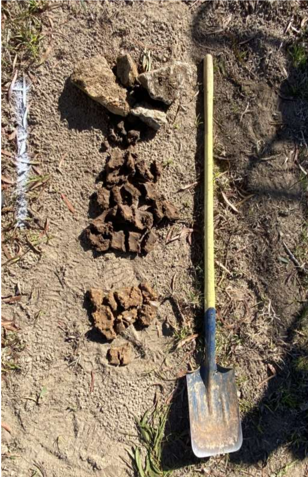
Figure 5: General profile of BH03 to 2m depth. Note large cobbles used as fill materials, likely to bridge underlying geotechnically unsuitable silts.
