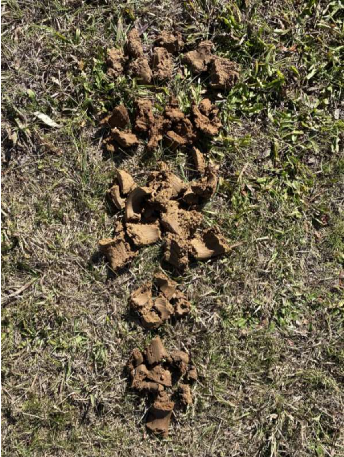
Figure 8: General profile of BH04 to 3m depth showing high plasticity alluvial clays directly adjacent to Muttama Creek and existing road culvert.
